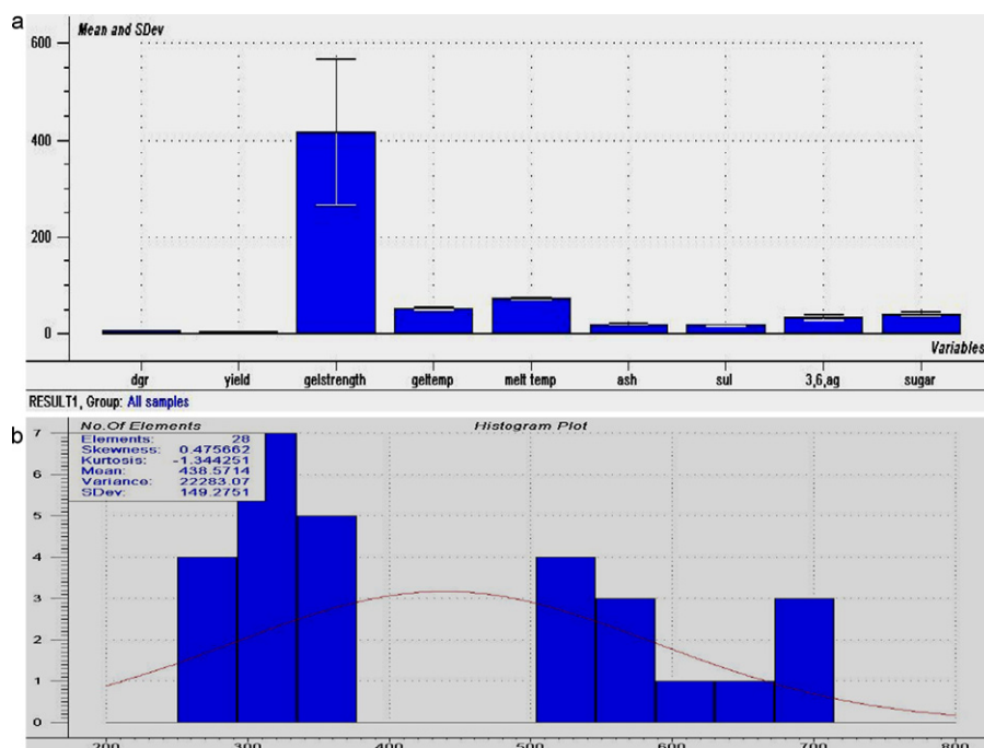
Fig. 5. (a) Mean and standard deviation among gel properties; and (b) histogram plot showing the values of mean and standard deviation of gel strength.
